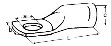
Cable lugs made of tinned electrolytic copper tube, without inspection hole according to DIN 46235. KHD is a cable lug produced according to German standards and, like KRT cable lugs, also fits compressed conductors (class 2), often used in the ship and offshore industry. KHD cable lugs are larger in terms of material and take up somewhat more space at the connection point.
