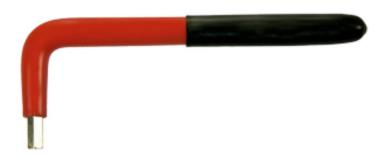
1000V ISOLATED UNBRACO. According to IEC 60900 Insulated tool with two-coloured and double-insulated handle for work on voltage up to 1000 V (AC). Visible insulation is red PVC in an anti-slip design that provides a good and secure working grip. When the insulation is damaged, layer 2 becomes visible (yellow colour), the tool is then no longer approved as an AUS tool. All tools are individually tested and labeled accordingly. Made in chrome vanadium steel.
